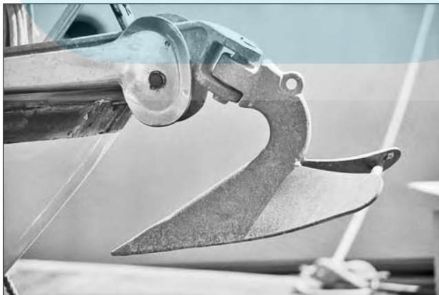
Figure 10-7: A plow anchor set in its roller on the bow, ready to go to work.
